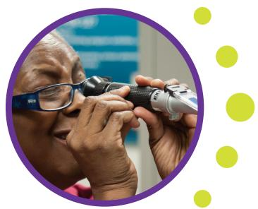
Top and Bottom: A refractometer is one way of measuring the salinity level of a water sample (Chesapeake Bay Program, Virginia Sea Grant). Middle: A probe can also be used for salinity readings (P. Bergstrom).
