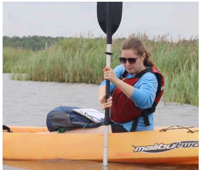
Press a paddle into the bottom sediment at a sampling site to collect data on sediment type. (Sky Swanson)
