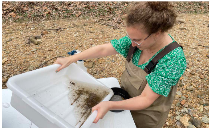
Pouring the contents from the white bin through the sieve concentrates the debris and organisms in the sample.
