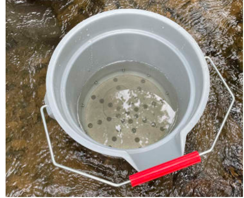
Sit the sieve bucket into the stream so that it is about half full of stream water.
