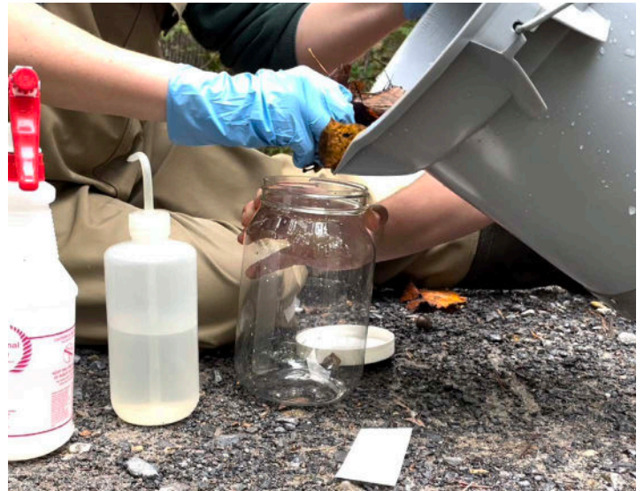
Using your hands, carefully move the bulk of the materials from your bucket into the sample jar.
