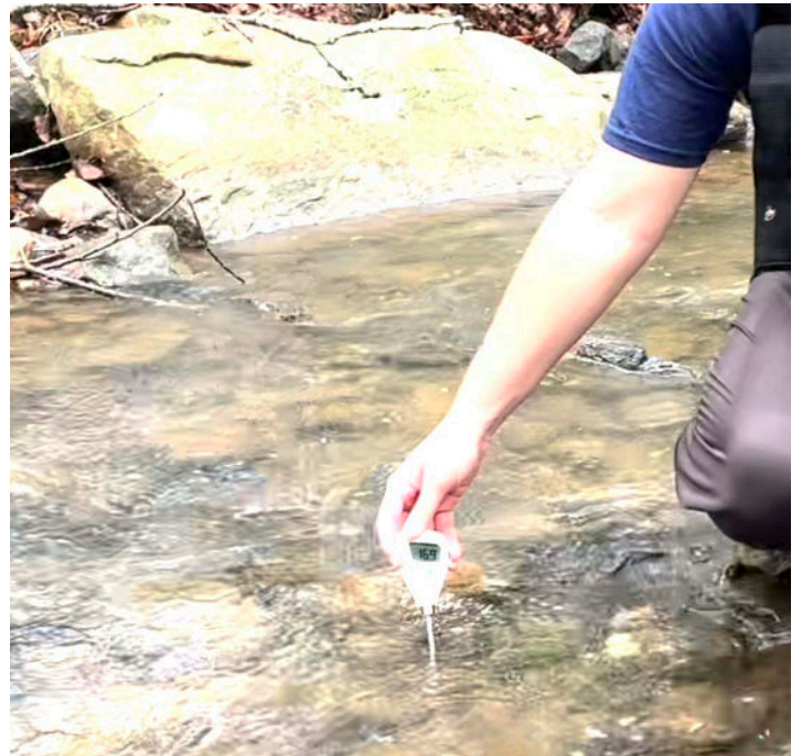
Take the water temperature in the middle of the channel.
