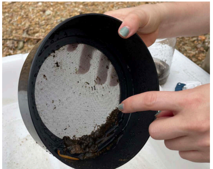
Once all of the contents of the bin are on one edge of the sieve, they can be more easily transferred to the sample jar.
