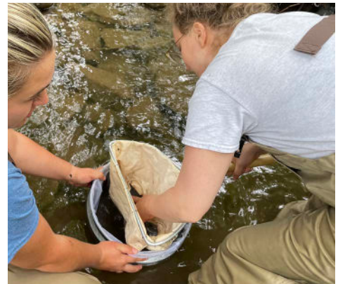
Dump the contents of the D-net into the bucket, turn the net inside out and rinse into the bucket. You can use a squirt bottle filled with stream water to help rinse.
