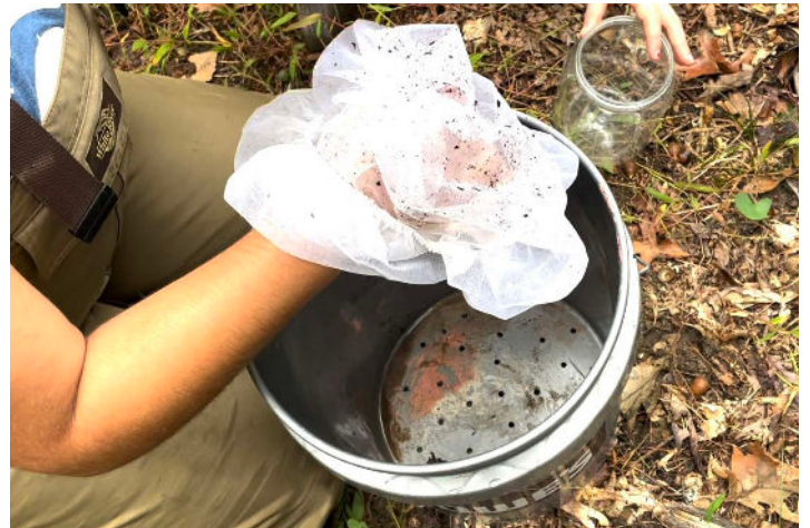
Roll down the sides of the bag over your hand. Turn upside down and gently push the bag into the sample jar.
