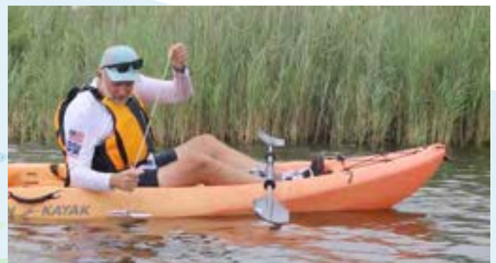
To measure water depth, lower the Secchi disk until it just barely rests on the bottom sediment. (Sky Swanson)
